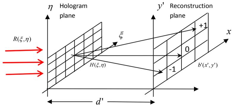
Fig.2. Reconstruction of a digital hologram
