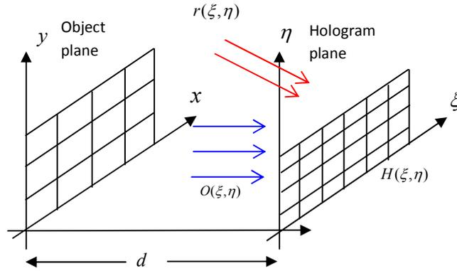
Fig.1. Recording of a digital hologram
